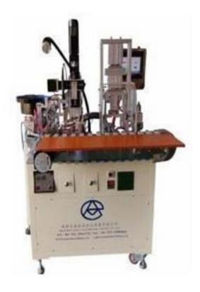
After earphone assembly it will be wounded and bounded by this machine and product will dispatch for packaging.
